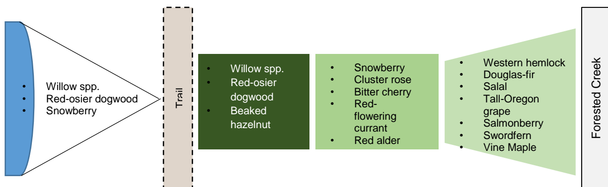
Figure 6: Plants were installed according to the site conditions. The east side of the corridor (right) has partial shade from the forested creek. The middle portion is dry and has full sun. The west section (left) receives full sun but is slightly wetter. The portion across the trail has very wet conditions.
